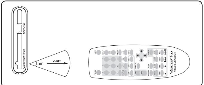
When using remote control, direct it towards the MEDIA-JUKEBOX within angles of 30 degrees +/- from the Remote Sensor at a distance of less than 24 feet away.
